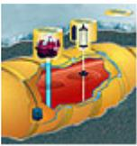
To comply with EPA regulations set forth in 1988, UPS removed, replaced or upgraded all of our underground storage tanks two years before the deadline at a cost of more than US\$100 million. Today we have approximately 1,056 total underground gas and diesel tanks in the U.S. These tanks utilize extensive protective measures, including leak-detection systems, redundant spill and overfill protection devices and built-in electrical interlocks and timers.
